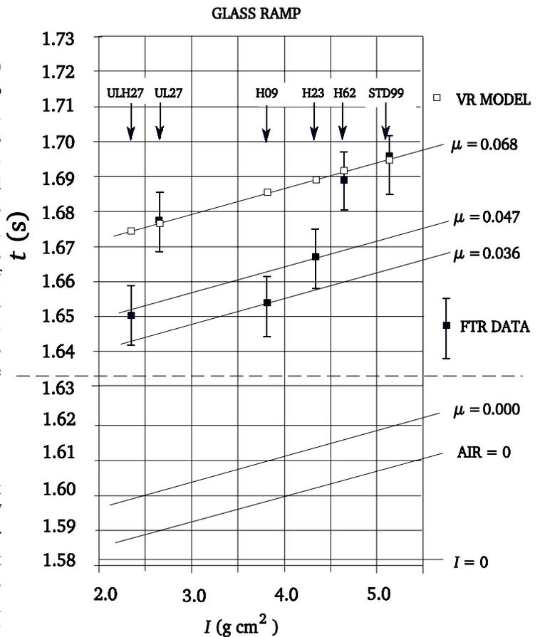
**Figure 2.** Showing results of different wheel sets run on the FTR with model data from the Virtual Race program.
