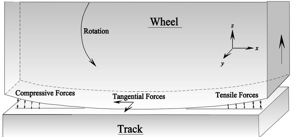
**Figure 4.** Perpendicular compressive and tensile forces in rolling friction.
