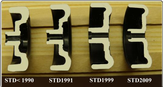
Fig 4 - Cross sections of all 4 wheels sanded and painted white for comparison.
