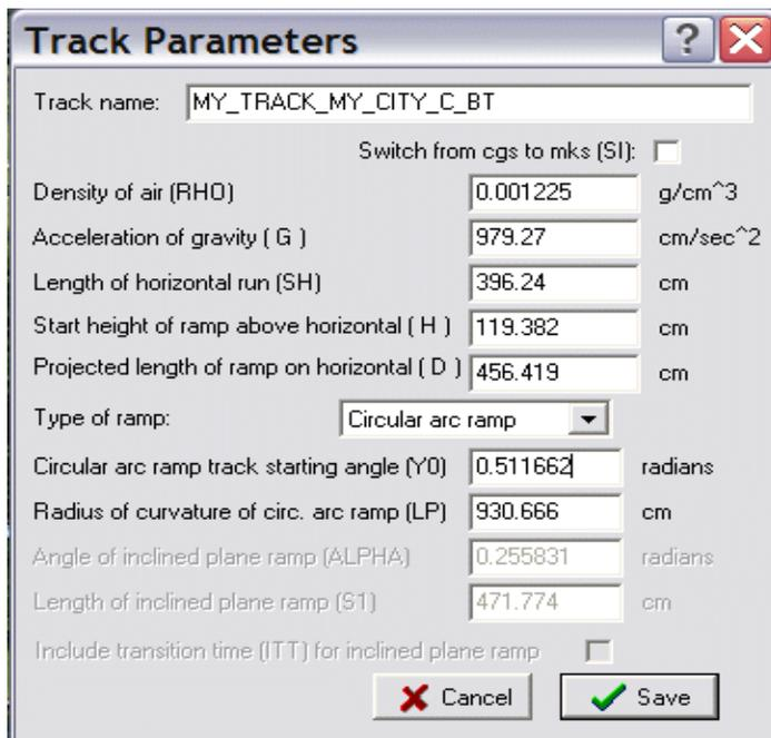
Fig 3 - Track with editable parameters that comes with the VR.
