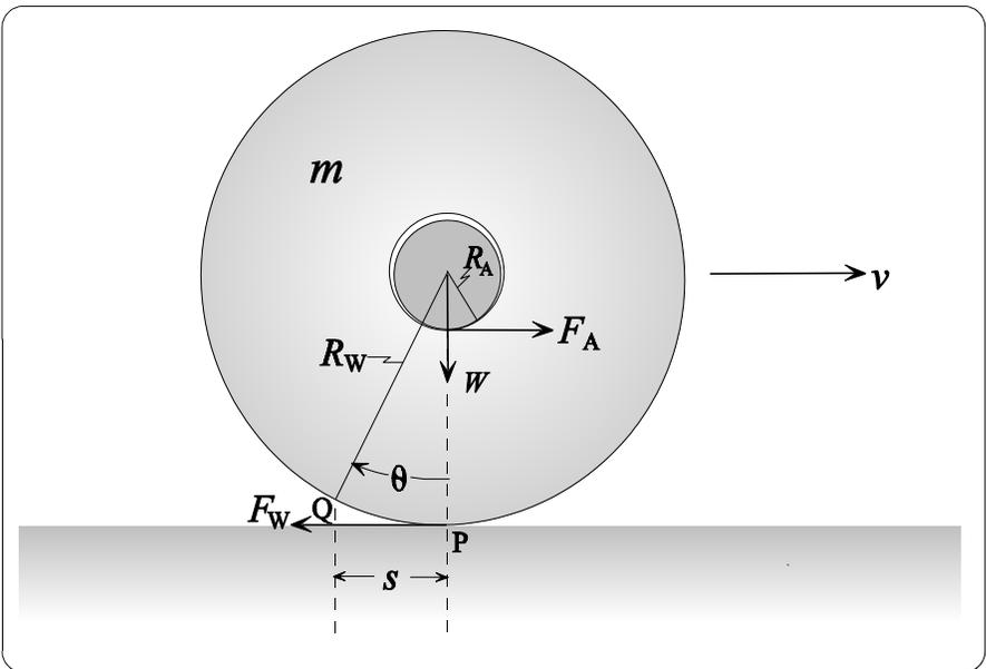
**Fig 6 - Forces and dimensions associated with a wheel.**
