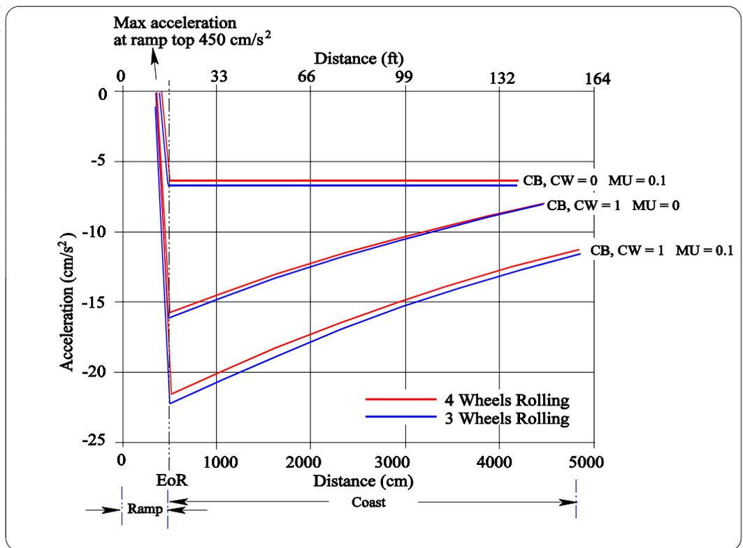
**Fig 10** - Using the [Display Results] feature of VR-II and Excel to examine coast accelerations.
