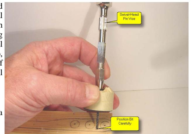
**Figure 5** - Hole starting with guide made from 2 wheels.
