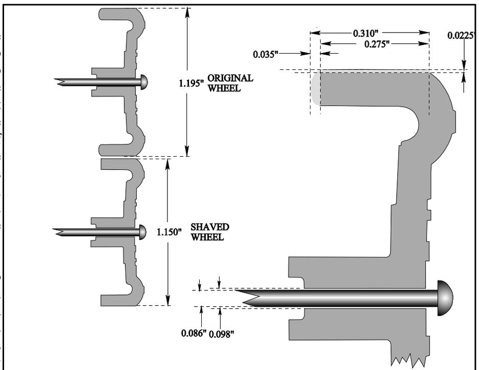
Figure 3 - Cross section of a 1999 BSA wheel showing wheel/axle specifications.
