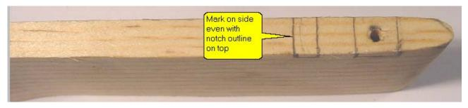
Figure 20 - Mark notch edges on sides of car.
