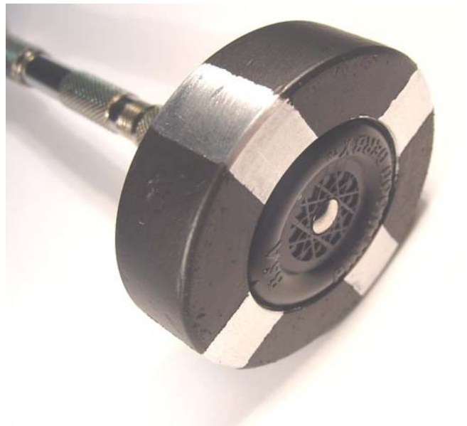
Figure 1 - Aluminum fitting FDS used to determine friction coefficients at different rotational velocities.
