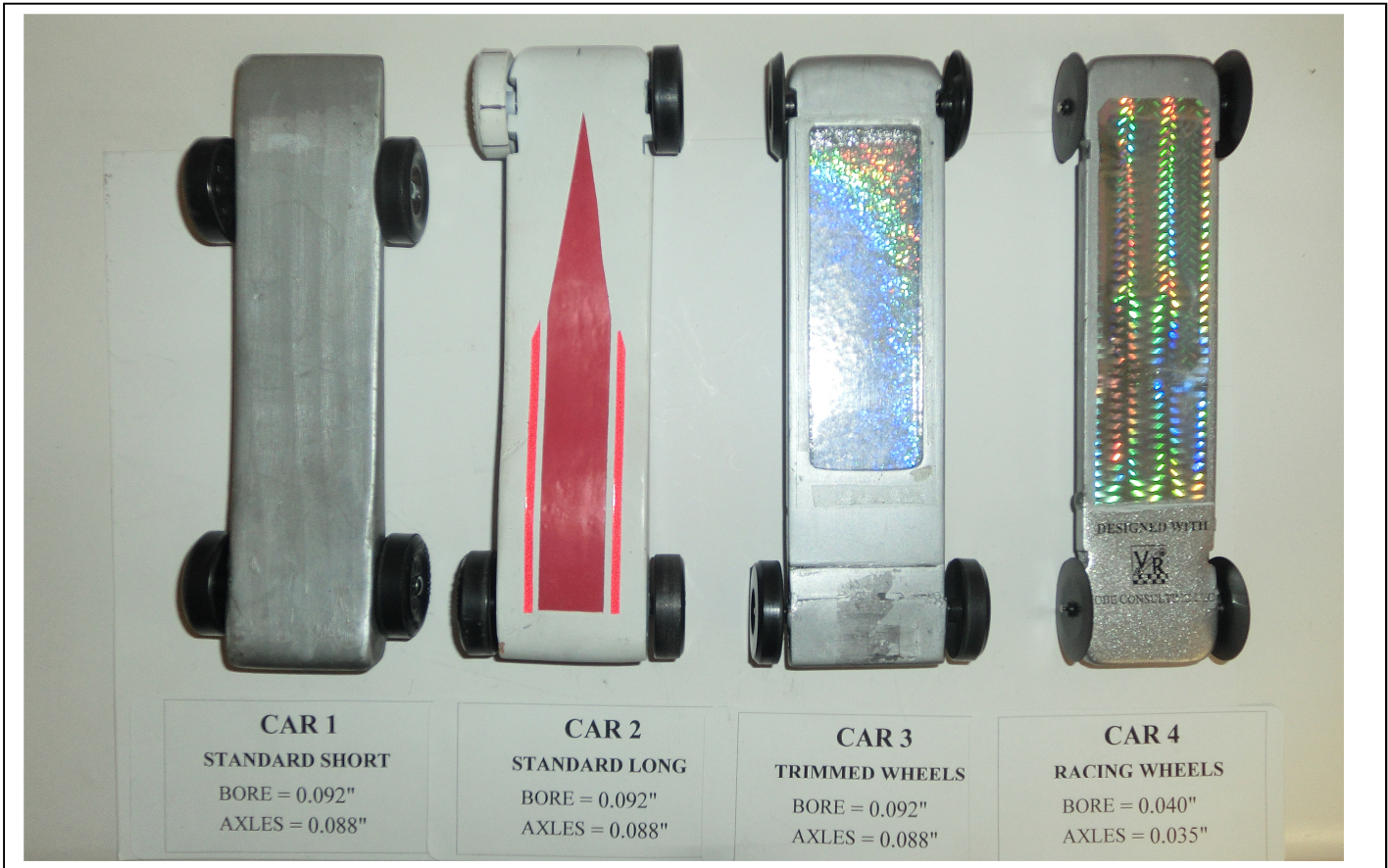
Figure 1 – The 4 Types of cars used in performance tests of the controlled-friction G-Track
