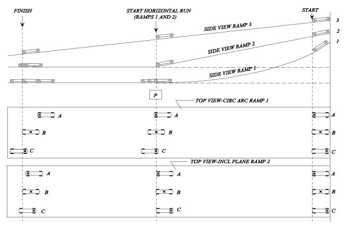
Figure 1 - Track 1 has a circular arc ramp, track 2 has an inclined plane ramp, and track 3 is all inclined plane.
