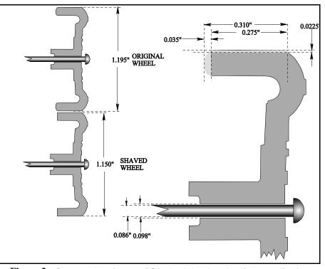
Figure 3 - Cross section of a 1999 BSA wheel showing wheel/axle specifications.
