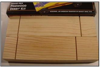
**Figure 4** - Slot spacing in blocks can be substantially different. Here the slots to the right vary by  $1/2^{"}$ .
