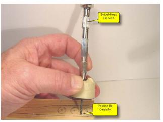
Figure 5 - Hole starting with guide made from 2 wheels.
