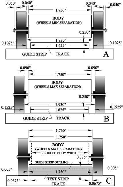
the 1-3/4" width rule with wheels at maximum separation (against axle heads), the wheels would be partly inside the 1-3/4" body. Nevertheless, as can be seen by the guide strip dashed outline, there would still be plenty of clearance, over 1/16", between the wheels and guide strip. Therefore, one will find many builders that will "notch" the body, or use a narrower body as shown by the vertical dashed lines or a really narrow body with wooden dowel spar extensions to hold the axle nails.
