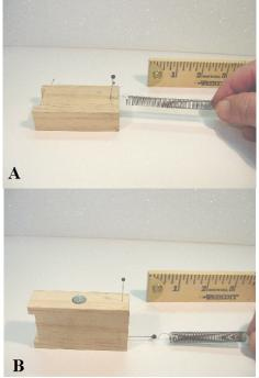
Figure 1. A - pulling a block with a block with a smaller area sliding.
