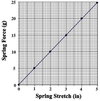
field). And it should also be noted that in pure Figure 4. Calibrating the spring of Figure 1 rolling of a hard wheel tread over a hard track there
