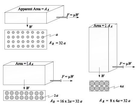
Figure 2. Sliding a block on 3 of its sides of different apparent areas.
