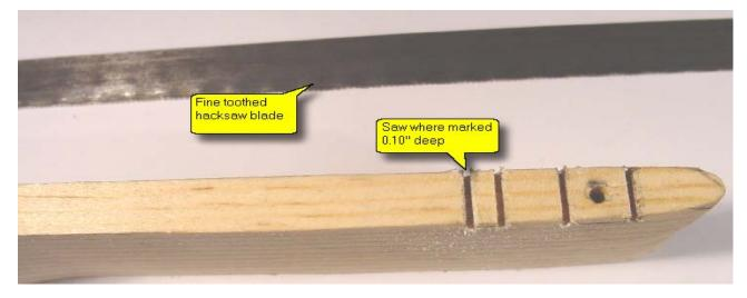
Figure 21 - Use a fine toothed hacksaw blade to cut notch edges on inside of pencil mark to 1/10 - in deep.
