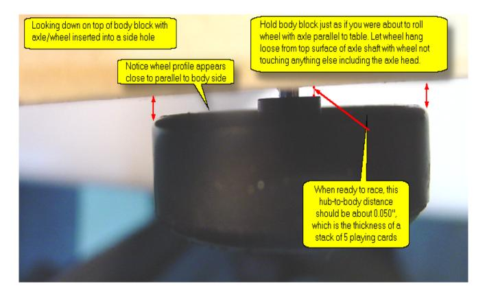
Figure 7 - Checking if the axle hole is perpendicular to the body sides.
