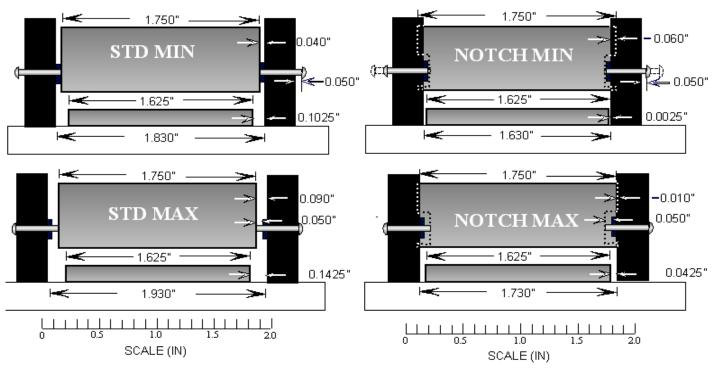
**Figure 19** - 4 views that explain why notching helps make for faster finish times. The rear wheels will follow the front ones provided the wheel tread surface is dry and free of graphite.
