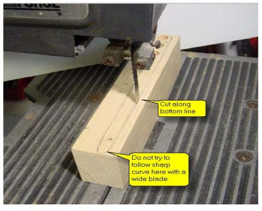
Figure 10 - Saw cut along car bottom trace
