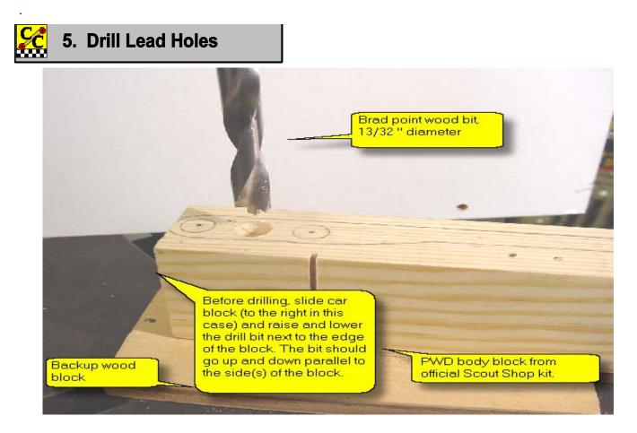
Figure 8 - Drilling the 13/32" holes for the 3/8" lead burning bar ( or "worms"). A 27/64" bit will also work.
