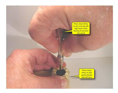
Figure 6 - Drilling the axle hole
