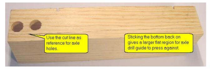
Figure 12 - Sticking the bottom piece back on
