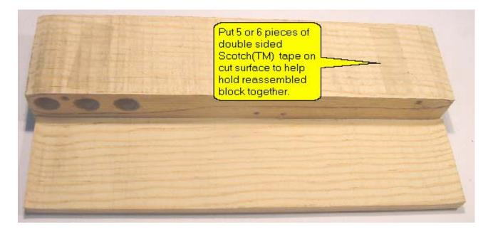
Figure 11 - Preparing to stick the bottom piece back on
