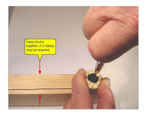
Figure 15 - Drilling the axle hole
