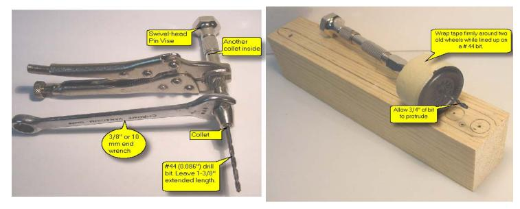
Figure 2 - Showing how to tighten a No 44 drill in the collet of a swivel head pin vise.
