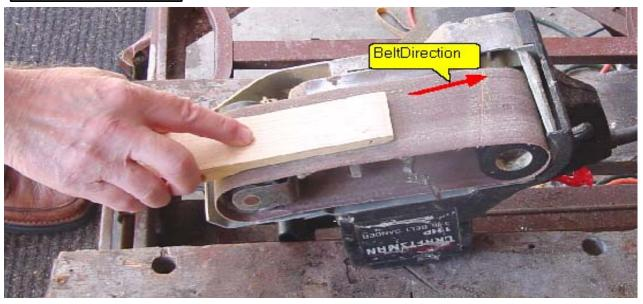
Figure 17 - Sanding the body with a medium grit.
