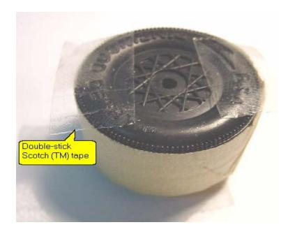
Figure 4 - Put double-stick tape on the drill bit guide.
