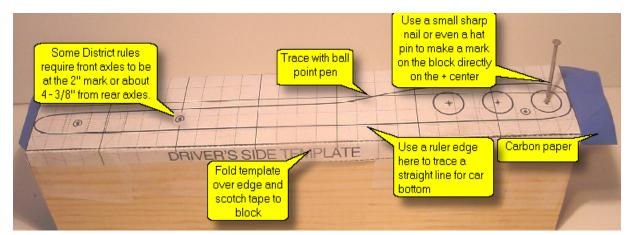
Figure 1 - The long wheelbase template from the next to the last page printed out and laid out on a standard kit body block over a piece of carbon paper. Check to make sure it is 7" long as printed.
