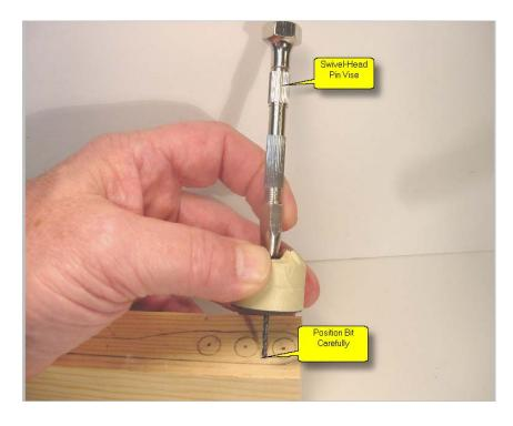
Figure 5 - Put double-stick tape on the drill bit guide.
