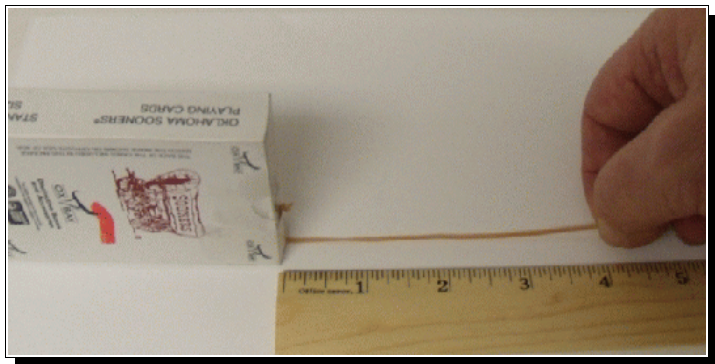
Figure 7 - Pulling the medium area and getting the average of 3 "stretch" measurements. Pinch thumbnail at 4 in just as rubber band lifts clear of paper,
