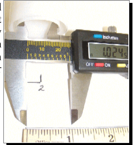
Figure 22 - Measuring roller ID as 1.02 in.
