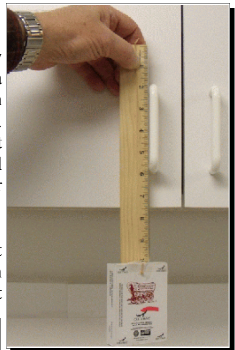
Figure 10 - Pinch the rubber band on the 1 in mark and raise the ruler until the deck starts to raise. Here the deck bottom has just cleared the bench top. Note the stretch distance on the ruler. Make sure the rubber band is a # 19.
