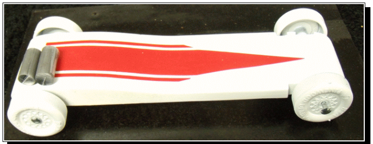
Figure 31 - Pinewood Derby car, lead weight distribution moved closer to right rear wheel.
